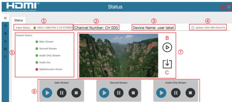
**① Input Status:** The status and information of the input signal. The green dot indicates that there is signal input, the format of the input audio and video is 720P60 dual-channel stereo. If the dot is red and shows "No Signal", it means there is no signal input.
