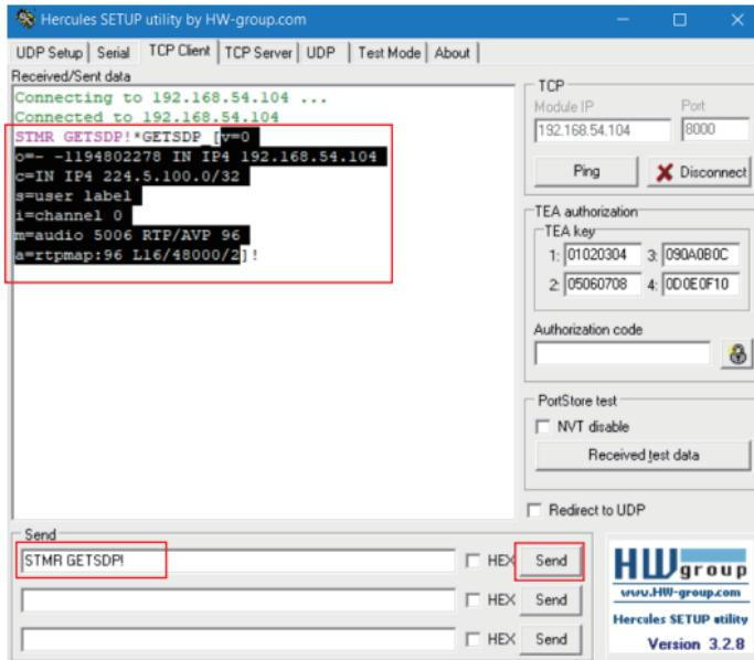
**Step 4:** Copy the obtained configuration file (selected part in the figure above), then paste it in the new-created notepad (or directly overwrite the content of the provided RTP\_AUDIO-STREAM-PCM.sdp file). Finally, save the file with the name of “RTP\_AUDIO-STREAM-PCM.sdp”, as shown below.
