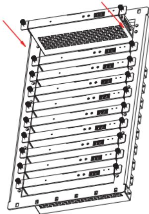
**Step 3:** Use screws to fix mounting ears on the rack to complete the mounting, as shown in the figure below:
