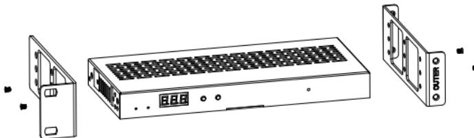
**Step 2:** Fix two rack panels on another machine in the same way, then fasten screws between two 1U V2 rack panels, so that two machines are mounted in a 1U V2 rack, as shown in the figure below:
